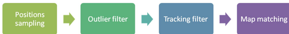
Figure 10. Processing steps for mitigating the positioning errors in user trajectory estimation.
